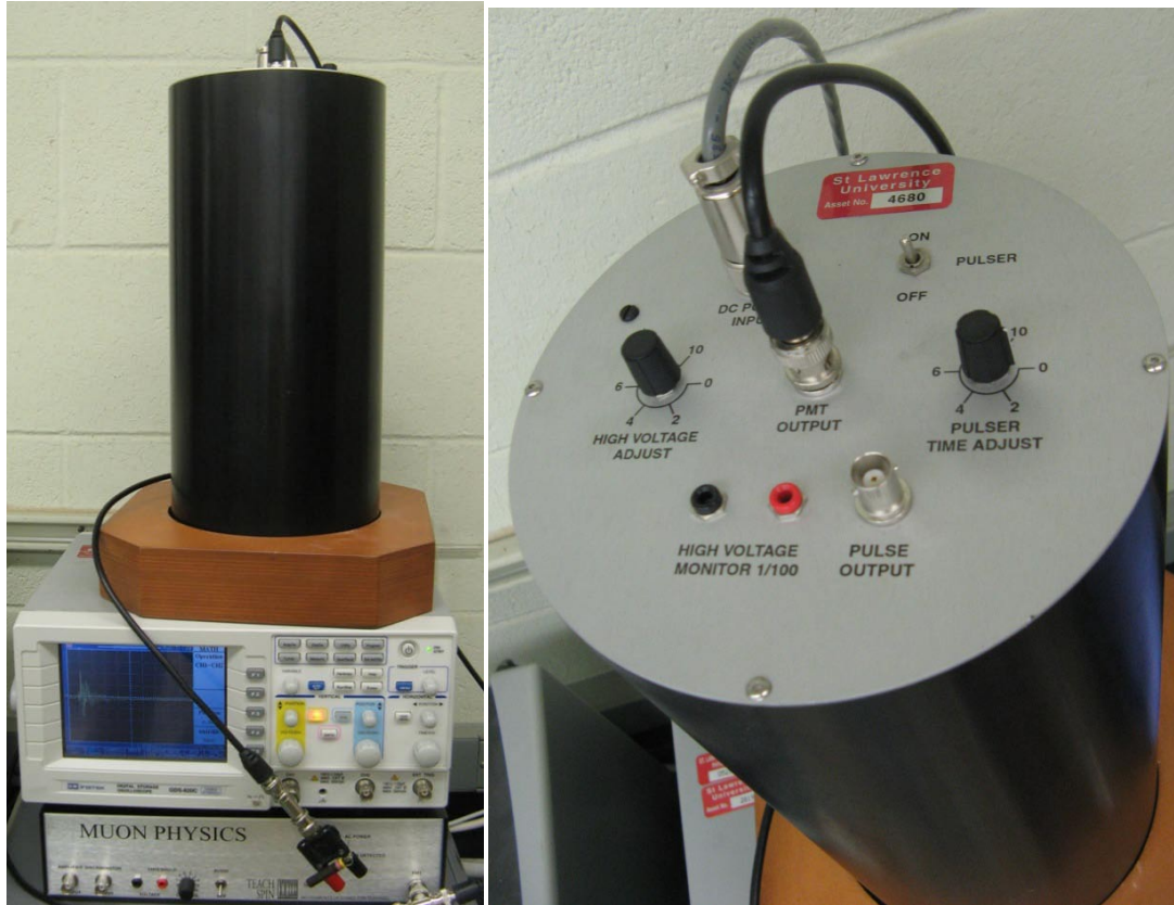
Left: Scintillator assembly sitting atop the oscilloscope and Experimental Control Unit. Right: Top of the scintillator assembly.
