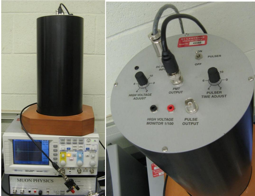
Left: Scintillator assembly sitting atop the oscilloscope and Experimental Control Unit.
